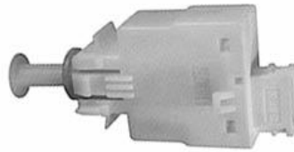
SL198 BMW 318i clutch pedal switch
